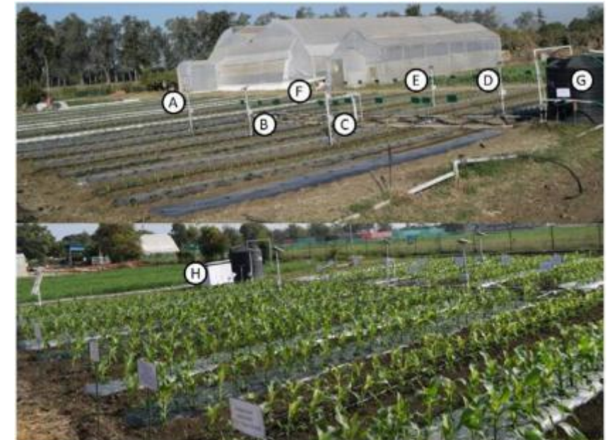
A, B, C, D, E and F: Data acquisition units, G: Pump and Tank section, H: Receiver section with 8 integrated relay module
